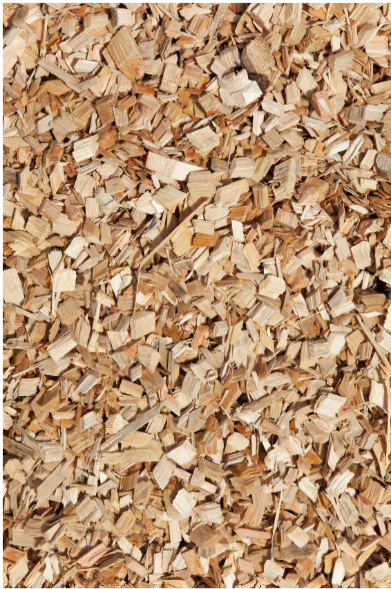
Wood chips can be burned directly for heating and electricity, converted into biofuel, or pulverized into powder to make wood fuel pellets.
